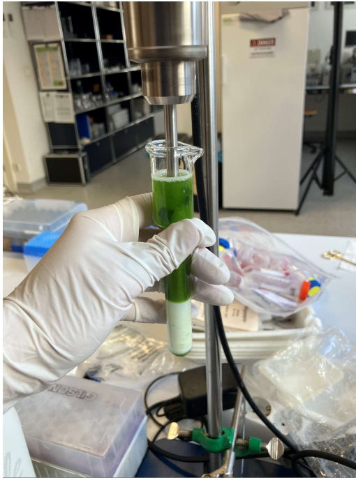
Figure 3: Homogenization of the cut leaf pieces.
