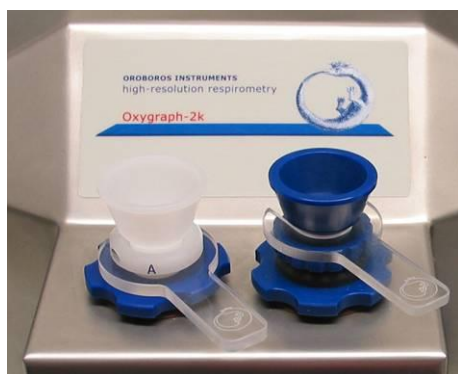
Fig.1 Stopper-spacers used for air calibration with the PVDF stopper (Chamber A) or titanium stopper (Chamber B).
