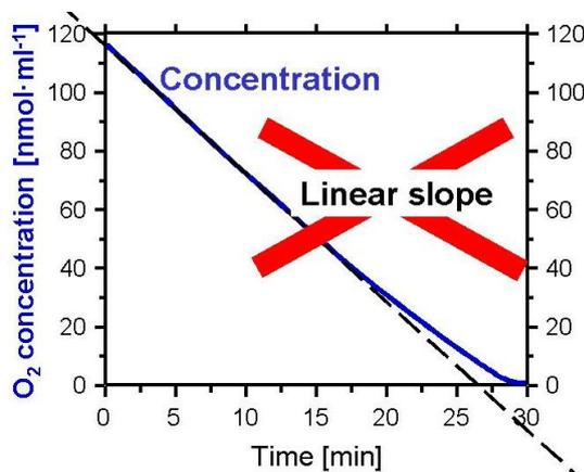
Conventional oxygraphic instruments display merely oxygen concentration over time, and oxygen flux (respiration) is estimated from the linear slope. Traditionally, linear sections of the experiment were analyzed using a ruler on the trace of the chart recorder. With this "eye-fitting" technique, traces appear to be more linear than they are. The "linear slope" approach belongs to the past of bioenergetics.
