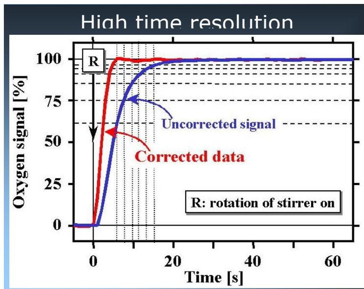
Sensors respond with a time delay to rapid changes of oxygen (uncorrected signal). Is the oxygen sensor sufficiently fast for kinetic studies? DatLab yields the answer, gives the exponential time constant and displays the time-corrected data (modified after Gnaiger 2001).
