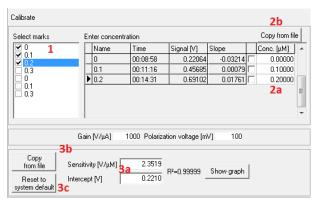
In the left panel the current calibration is shown. The right panel is used for a new calibration. Select the marks to use for the calibration (1). The column "Conc." will be filled automatically with the "values" associated with each mark, MiPNet19.19. see Alternatively, the known enter concentrations manually (2a) or
