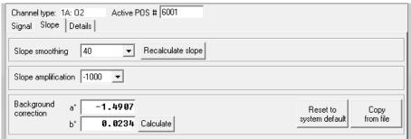
Slope smoothing ▼ Select the number of data points (*N* = 40 to 5 in intervals of 5) used to calculate the slope through a polynomial fit, as a basis for the plot of flux. A high value of *N* yields a highly smoothed curve, whereas a low value of *N* improves time resolution. Apply with Recalculate slope or Calibrate and Copy to Clipboard. It may take time to recalculate the slope.
