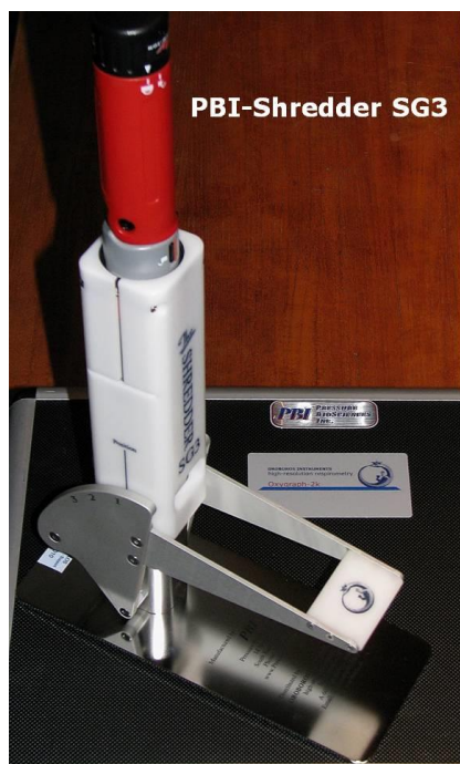
Figure 1: The PBI-Shredder SG3 with handle (red) and torque driver (white) assembled with the force setting lever (metal) ready for application.
